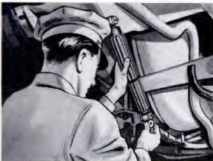
This is a view of a typical rear end shock absorber installation. At the top of advertisement on the right, you will see a typical front end shock absorber installation.
